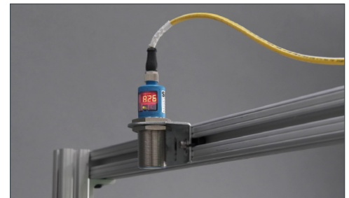
Height sensors allow the Servo Stand to automatically adjust for the next product in the label production line by measuring overall height of the product.
