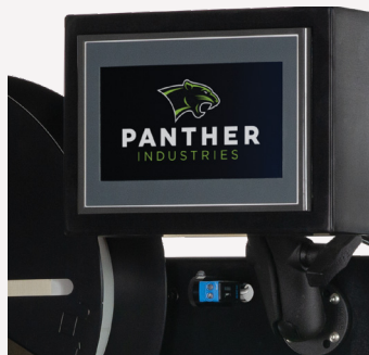
Remote-mounted 7" touch screen display, and low label sensor.
